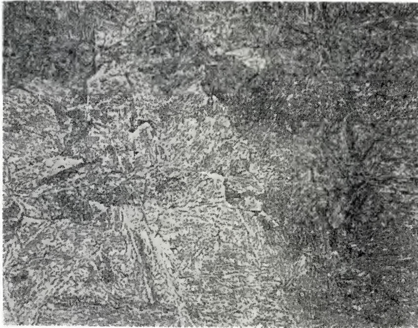
FIG. 4 - Microstructure at mid-wall of reheat treated rotary forged hollow ESR cylinder (Top) - 100X (See Table 2)
